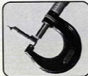
Use a micrometer to measure the amount of metal filed to reduce sear engagement.
