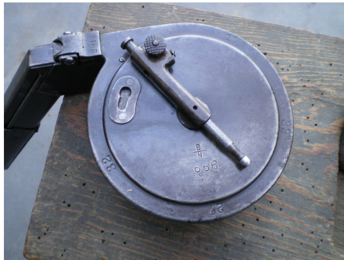
2a. Bing Brothers Telescoping Crank Bottom Plate With Retainer Screws
