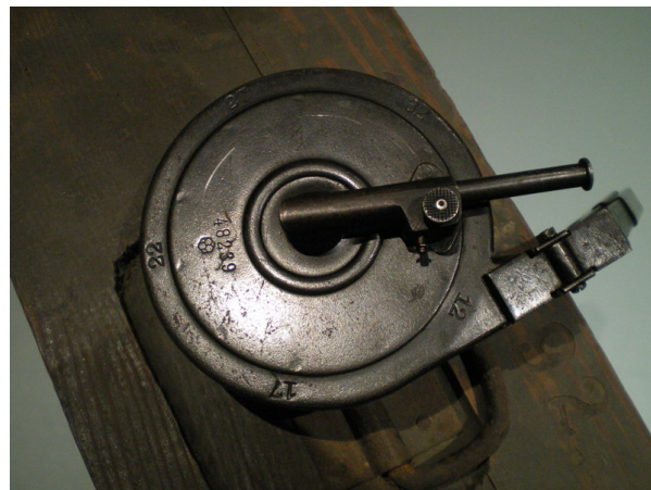
1a. AEG Telescoping Bottom Crank Plate With Reinforcing Ring.
