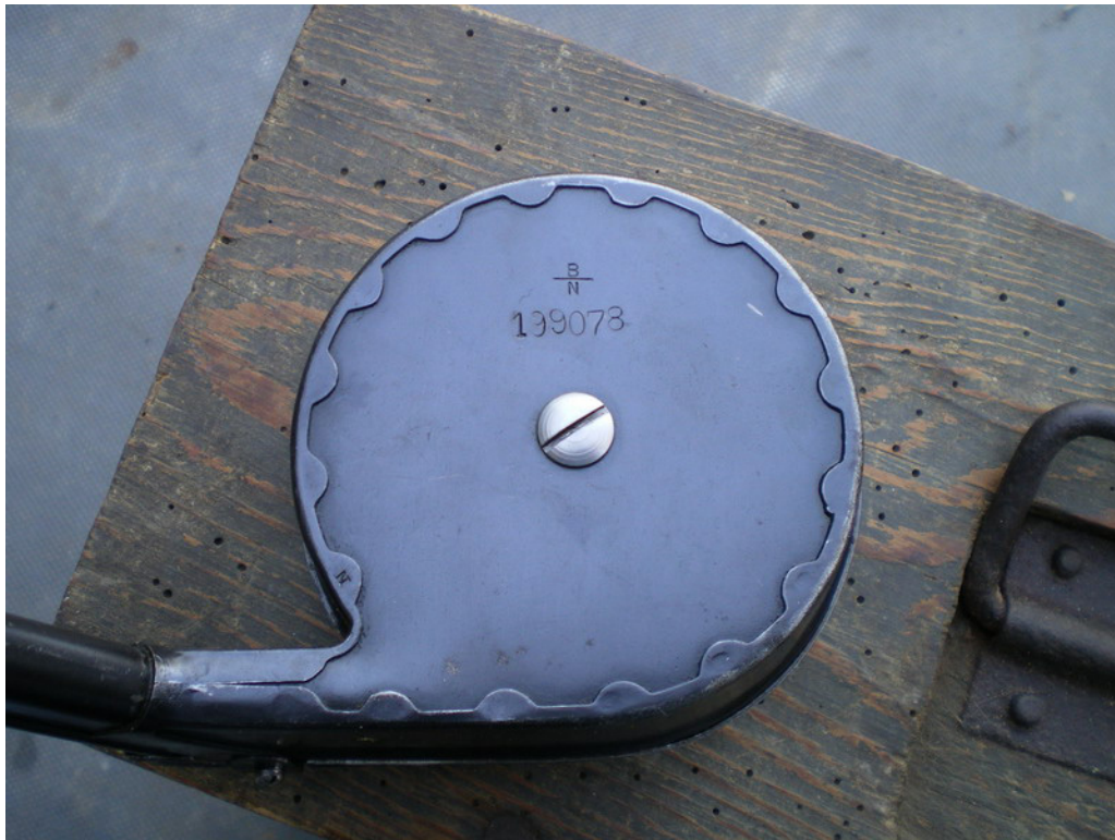
5b. Bing Brothers Folding Crank Top Plate
