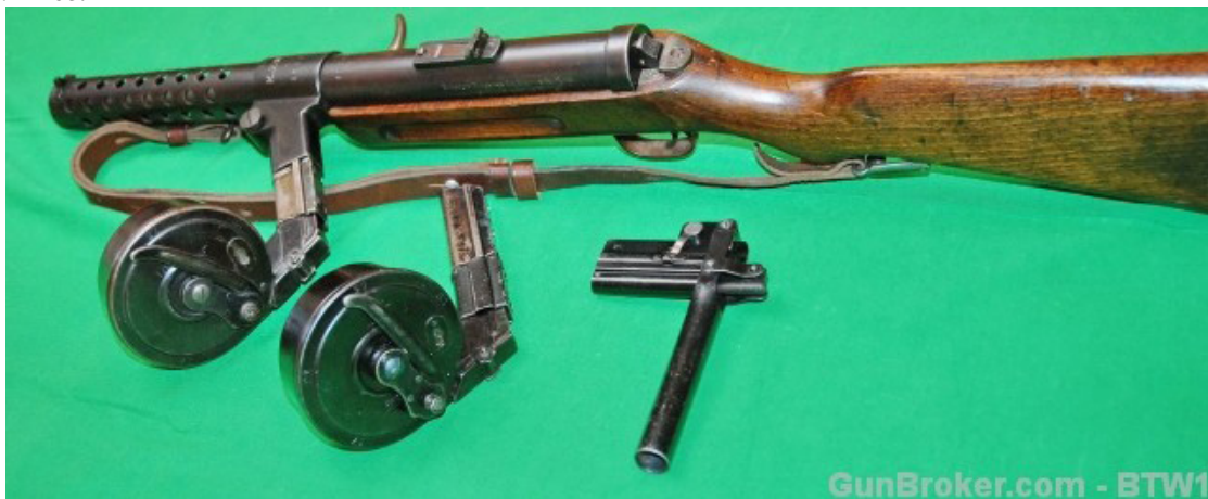
MP.18 With Trommel Magazine Note Adapter Position
