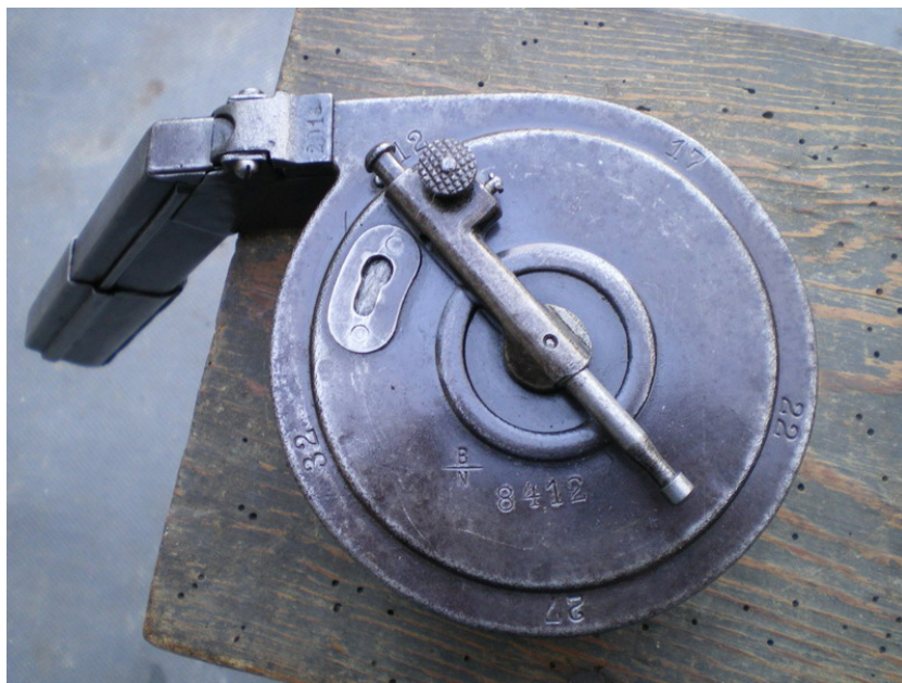
3a. Bing Brothers Telescoping Crank Reinforced Bottom Plate With Retainer Screws
