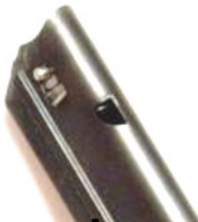
Trommel Magazine Stem Neck Hold Open Pin & Locking Groove
