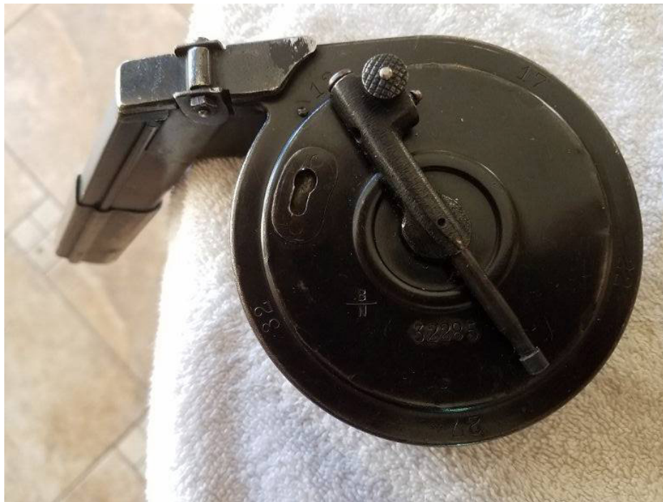
4a. Bing Brothers Telescoping Crank Bottom Plate With Retainer Through Bolt & Nut
