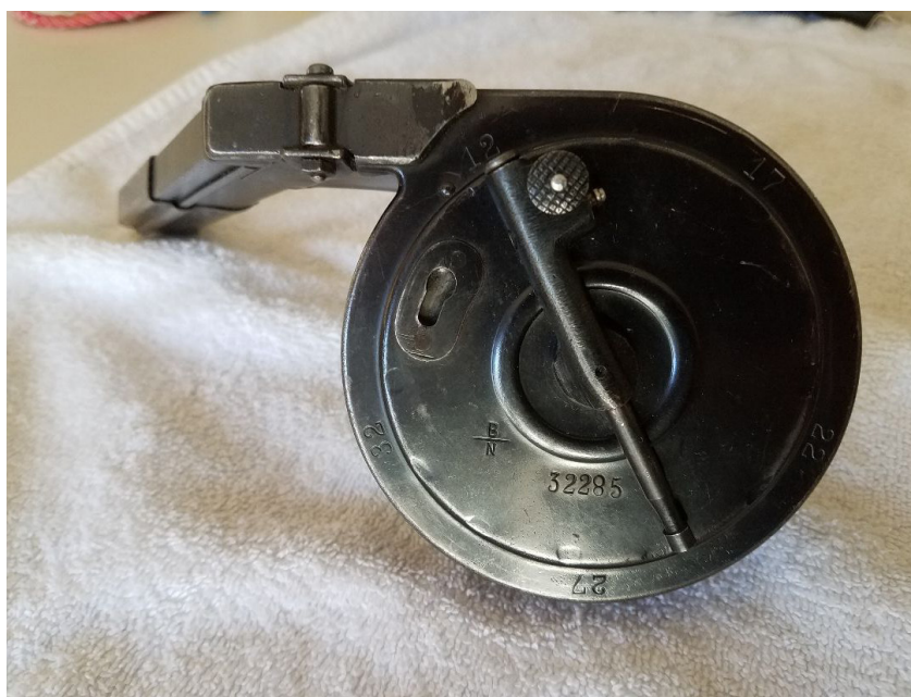
The Sliding Steel Pin Winding Lever Early TM.08 Variation
