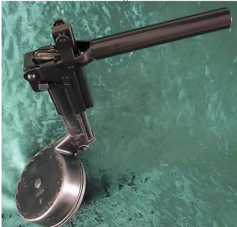
Magazine With Loading Tool Attached
