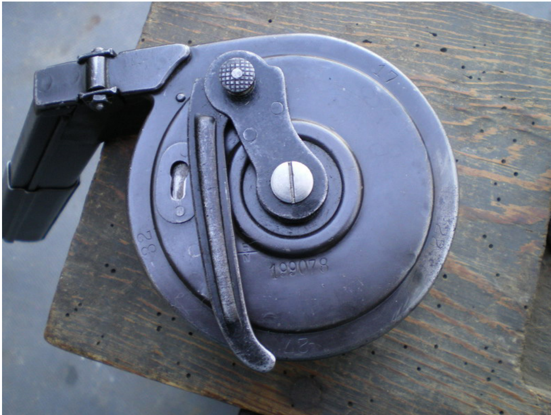
Trommel Magazine Folding Winding Crank Lower Plate Features.
