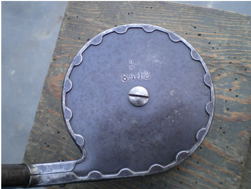
3b. Bing Brothers Telescoping Crank Unreinforced Top Plate
