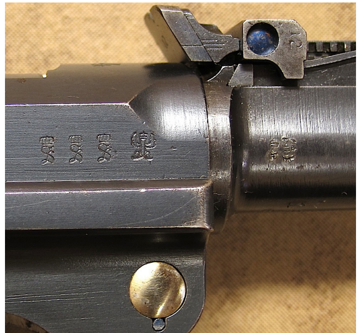
1914 DWM LP.08 C/S Acceptance And Reichsadler Proof Marks On The Receiver And Barrel.
