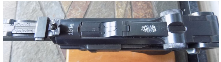
1914 DWM LP.08 Top View With Rear Tangent Sight Fine Adjustment Screw Head.
