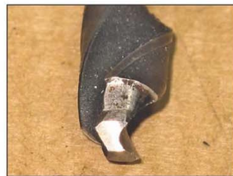
Photo 12. Cutting face backed off.
