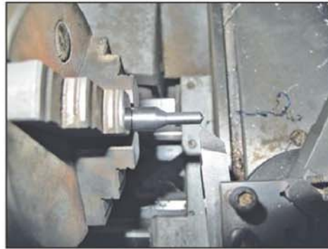
Photo 17. Turning 120 degree angles to D bit.
