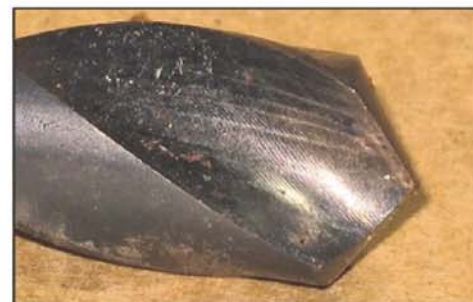
Photo 8. Drill before the web thickness reduction.
