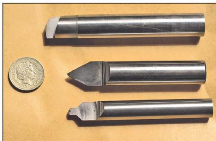
Photo 3. D bits ground from round HSS.
