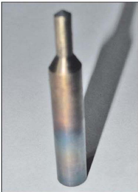
Photo 21. Tempering colours run from heat source at the base. Cutting faces achieving light straw colour.
