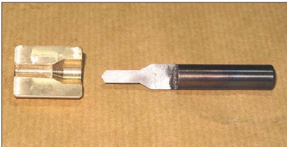
Photo 27. The sectioned cut with the cutter that made it.
