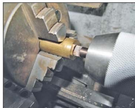
Photo 25. D bit plunged to full cutting depth.
