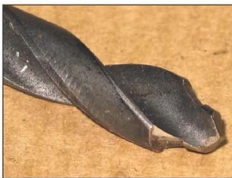
Photo 11, a double diameter form drill, with 45 degree blend face.
