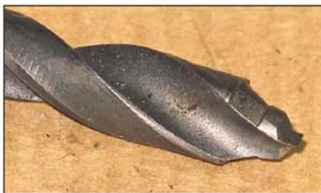
Photo 13. Web thickness reduction.
