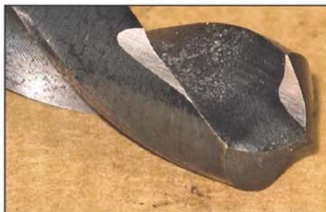
Photo 9. Drill after the web thickness reduction.
