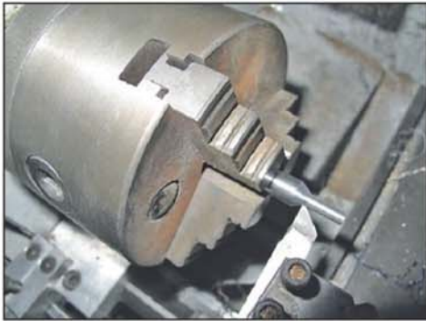
Photo 16. Turning 60 degree angles to D bit.
