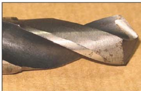
Photo 7. Double diameter drill, showing hand ground backing off, to leave a cutting land. The web thickness has also been reduced.
