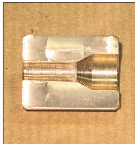
Photo 26. Sectioned view of plunged cut.
