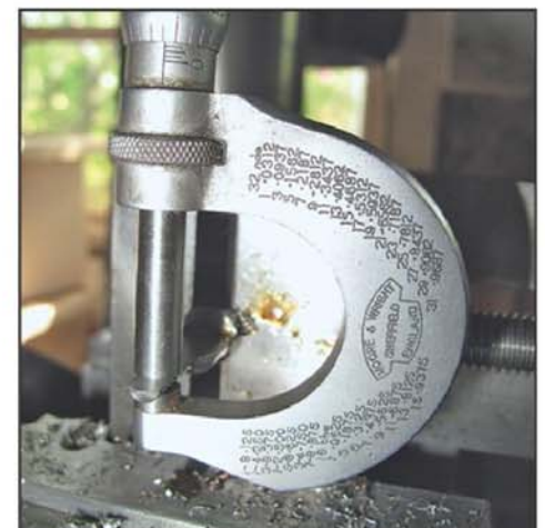
Photo 20. 0.1875in. diameter milled to centre line, leaving 0.002in. for finish stoning.
