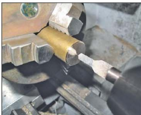
Photo 24. Proving D bit by plunge cutting
