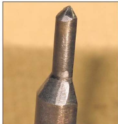
Photo 23. Backed off cutting faces.
