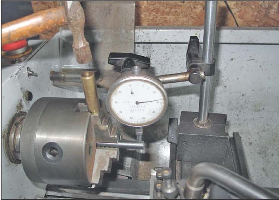
Photo 15. Set stock true, by gently tapping chuck jaws.
