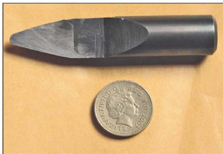
Photo 1. Silver steel "D" bit, milled to centre line, hardened and stoned to achieve smooth cutting edge.
