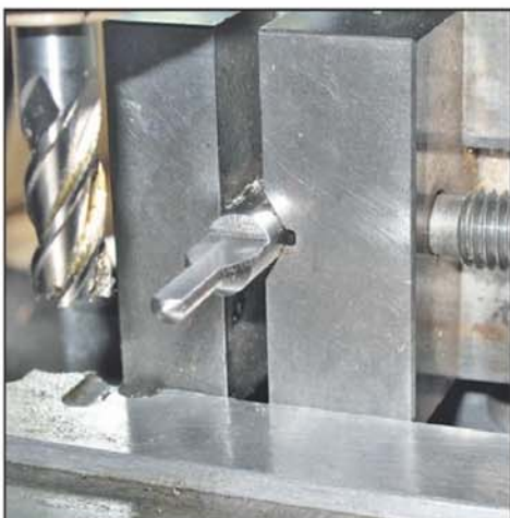
Photo 18. Milling D bit to centre line.
