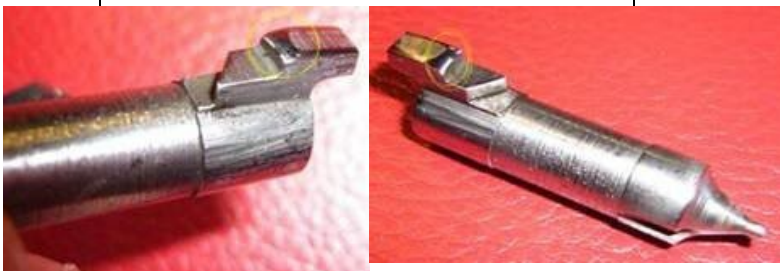
STRIKER HELD WITH WORN OR IMPROPERLY FINISHED SEAR
