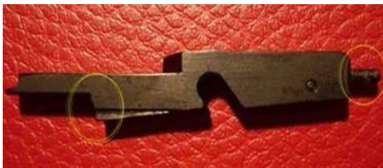
SEAR ANGLE CUT SHOWING ABUSE AND WRONG DISCONNECTOR PLUNGER BUTTON
